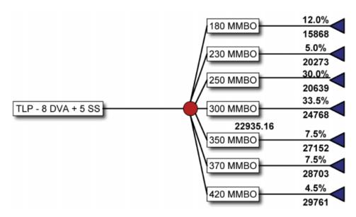
Fig. 5—Expected value of base case design of development with probabilities for OOIP.
