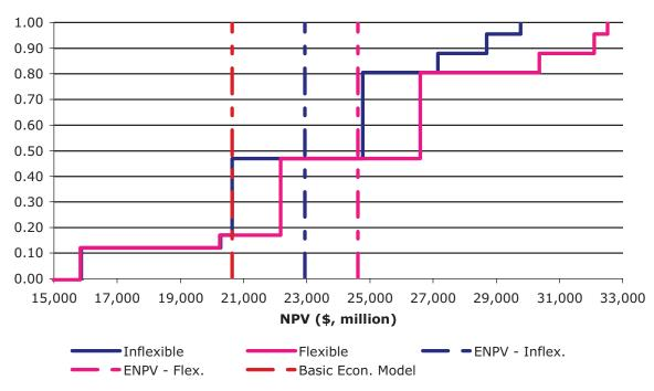
Fig. 9—VARG curves comparing the development of the combined fields with and without flexibility. Dashed lines show their ENPV.
